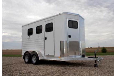
Aluminum Roof, Walls, Cross members
