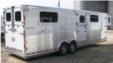
Full-length Aluminum Side Extrusion
