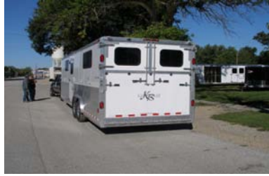
Aluminum Roof and Exterior
